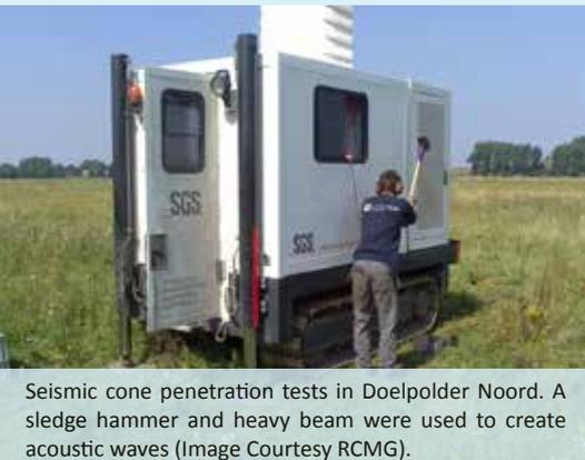
Seismic cone penetration tests in Doelpolder Noord. A sledge hammer and heavy beam were used to create acoustic waves (Image Courtesy RCMG).
